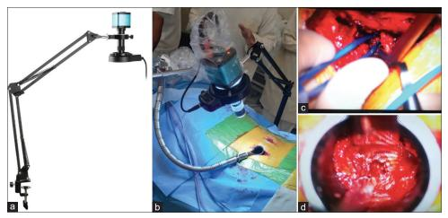
**Figure 1:** The fully assembled low-budget exoscope (a) composed of video microscope camera, C-mount lens, LED ring light, and cantilever. Intraoperative setup (b) with camera pointing at tubular retractor in a minimally invasive transforaminal lumbar interbody fusion (TLIF) procedure. The surgical field of an open TLIF (c) and a minimally invasive TLIF (d) as projected on the television screen.
