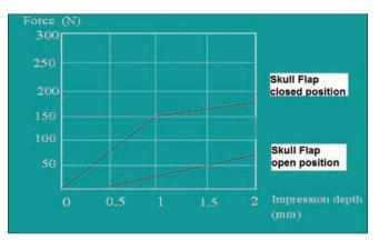
**Figure 7:** Graphic showing the load-bearing test on SF device demonstrating that it is needed 70 N = 70 kg of impression force to make 2 mm descent of the bone in an open position as well as 175 N = 175 kg of impression force to make 2 mm descent of the bone in a closed position
