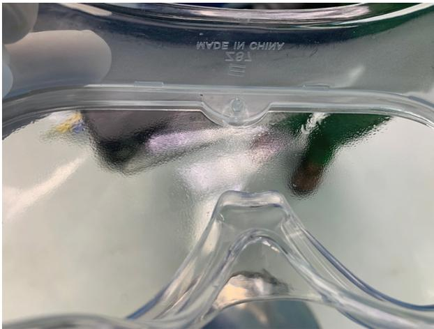
**Fig. 2** Goggles with antifogging coating have the phenomenon of forming a fluid layer, which deteriorated vision by chromatic aberration.
