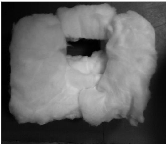
**Figure 3:** The thick cotton roll used on the device for a cushion effect
